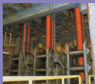
連続铸造設備 Completely vertical type bloom caster
