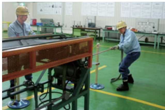
Experiential learning about being caught into a roller of a belt conveyor
