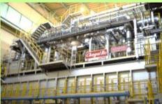
Energy-saving heating furnace that uses regenerative burners
