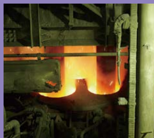
取鋼精錬設備 Ladle furnace
