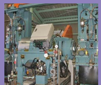
鋼管用水浸超音波探傷機 Water immersion ultrasonic inspection machine for steel tubes
