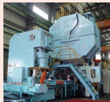
An additional 2,000-ton vertical-type press which installed at the formed and fabricated materials subsidiary in China.
