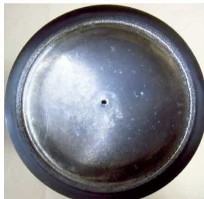
Fig.8 Surface appearance of the punch with a center air vent after 15000 shots.
