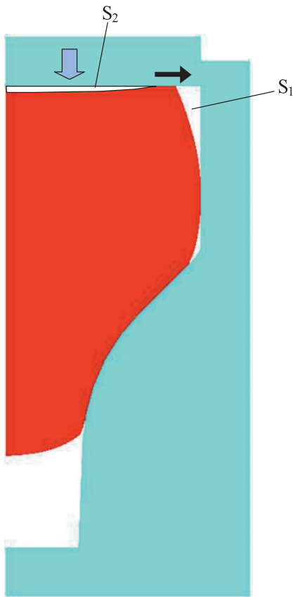
Fig.4 Schematic diagram of lubricant trapped room.
