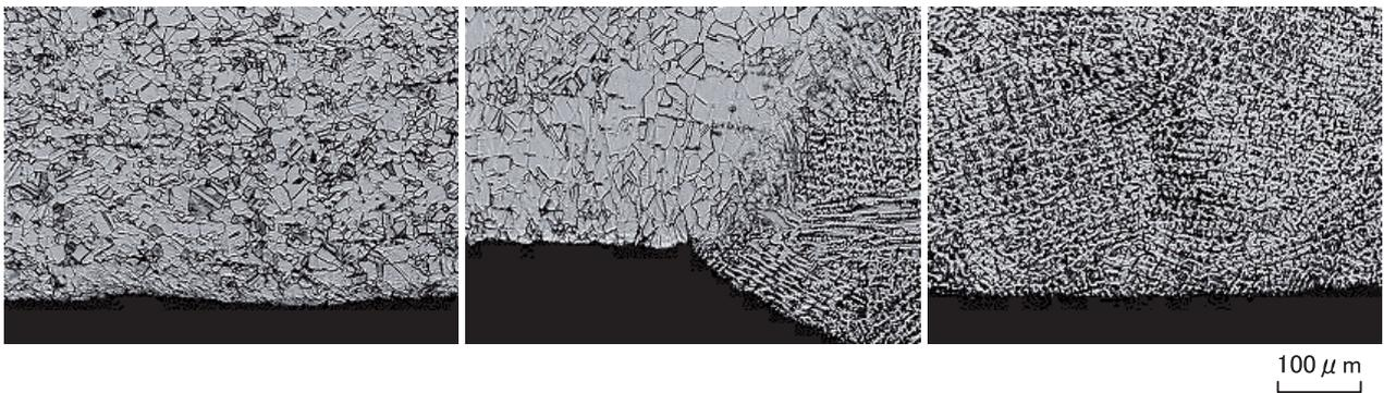
Fig.10 Microstructures of the weld joint.
